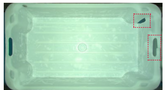
Automatic CIB control prevents circulation of boxes unfit for production
